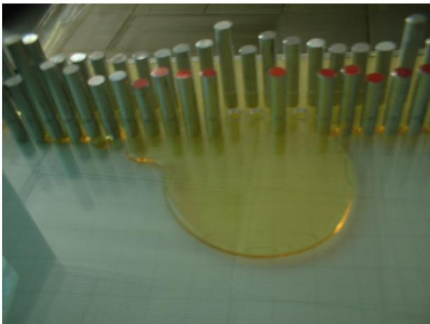
Figure 2: Physical model of a dislocation movement using an acrylic box, aluminum pegs, and glycerin.
