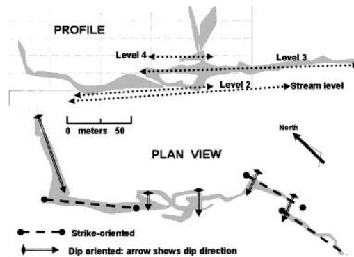
FIG. 7. Dimensional plan/profile map of Sistema Vientos. Strike and dip symbols are as in Fig 4.
